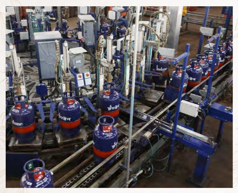
A view of IndianOil's LPG Bottling Plant with automated filling of LPG cylinders.
