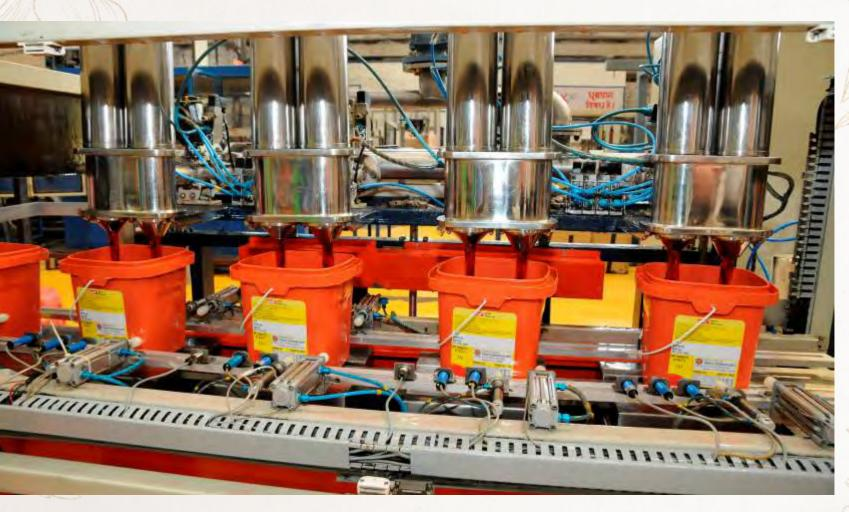
A view of the lubricant plant in which lubricant is being filled in containers by an automatic filling and packing system.
