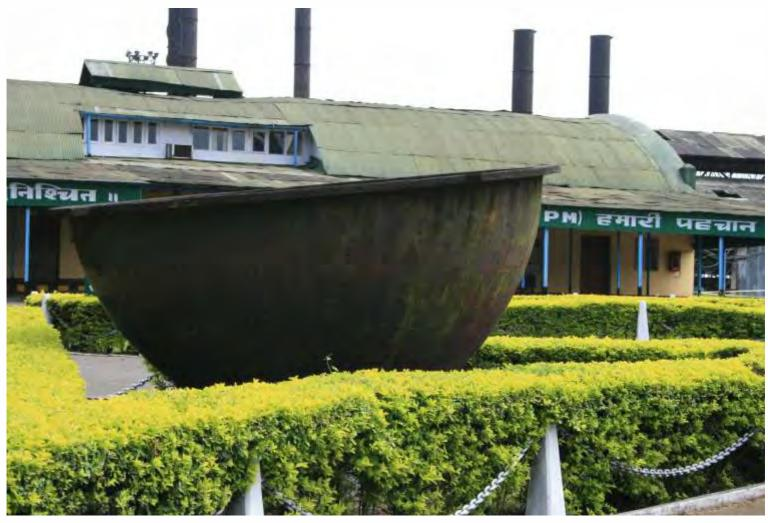
The century old Digboi Refinery's still, the equipment used for oil refining at the time.
